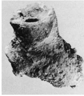
27. Fragmentary clay funnel for receiving bronze into mold. Restored drawing shows pouring channels (gates) through which bronze flowed from funnel into mold cavity.
