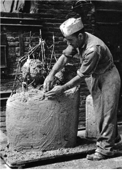
32-34. Lost-wax casting, although now refined in the details, is a process which has not changed significantly since antiquity. These views of a present-day foundry show the building up of a clay mold, a brick furnace much like an ancient one, and the pouring of bronze into funnels leading to molds packed in a makeshift casting pit. 1957.
